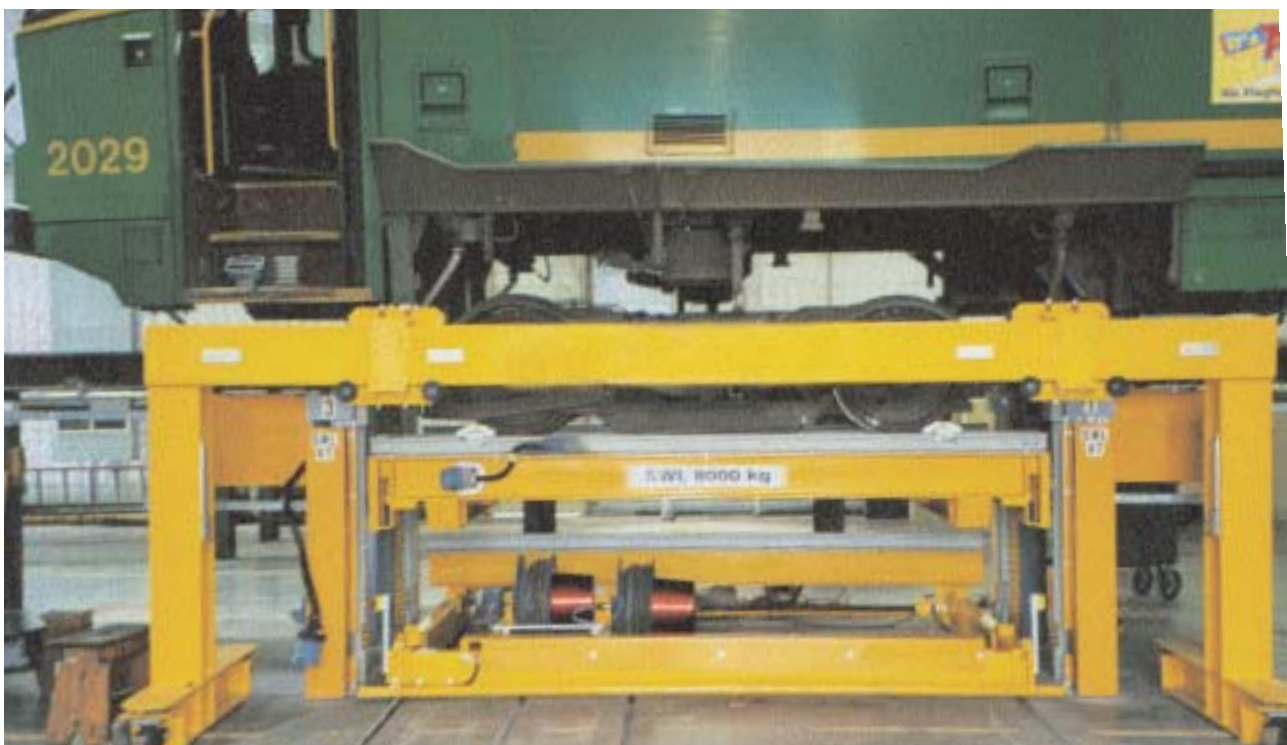
Above: Specially-designed and built bogie repair hoists at one of the Hong Kong Rail maintenance depots. Below: This unique bogie removal system was designed and installed for Yarra Trams, Melbourne (see opposite page for different view).
