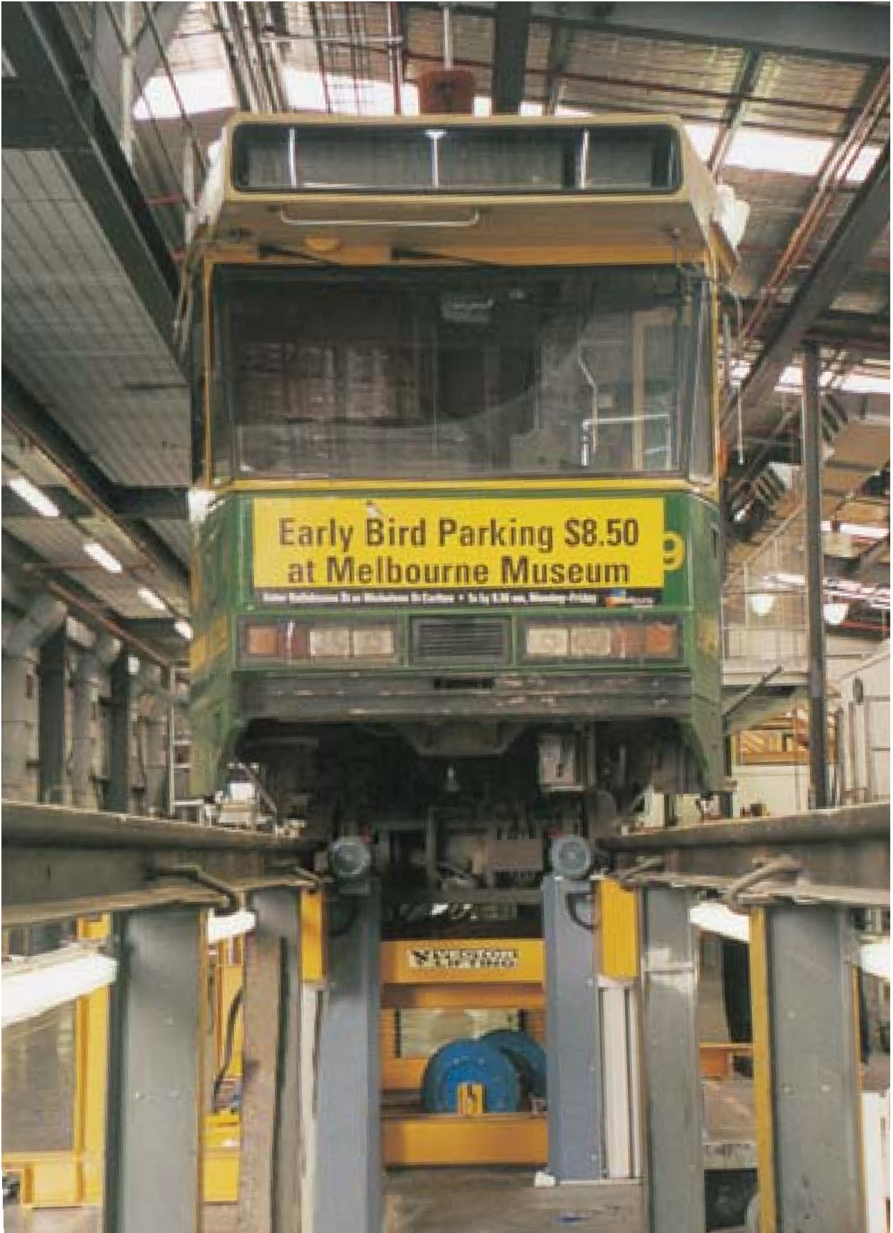
Vector's special bogie removal system for Yarra Trams facilitates maintenance and repair procedures.
