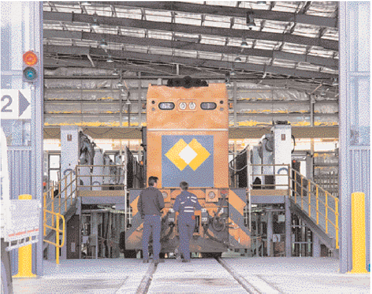
This locomotive is on a drop table at Spotswood, Victoria, undergoing maintenance work.
