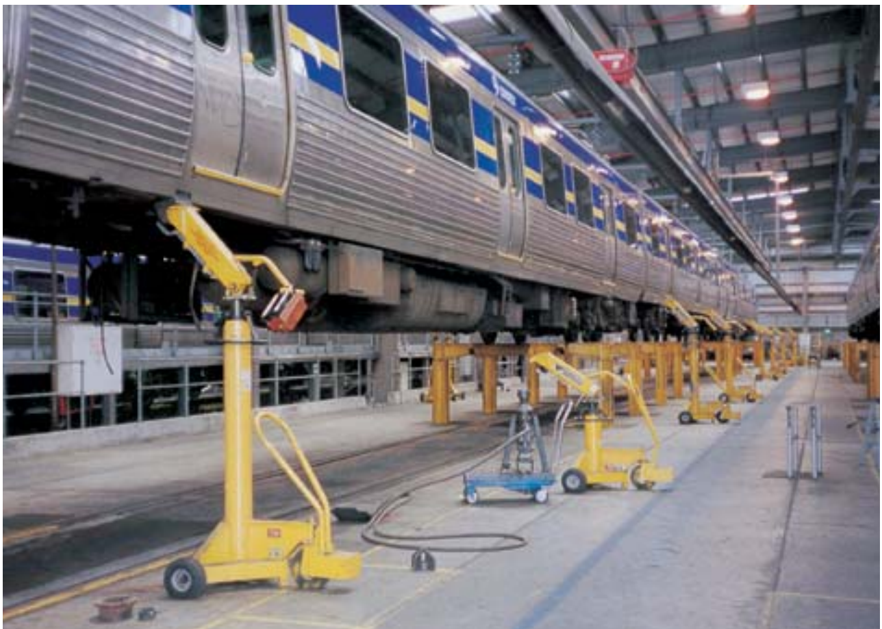
These photos were taken at the Epping service facility in Melbourne, Victoria and show Vector's four car under floor lifting system with special mobile body supports.
