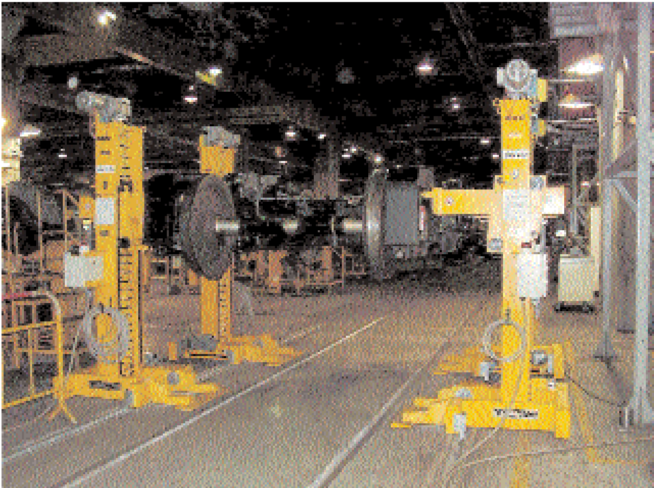
Above: Specially-designed and built bogie repair hoists at one of the Hong Kong Rail maintenance depots. Below: This unique bogie removal system was designed and installed for Yarra Trams, Melbourne (see opposite page for different view).
