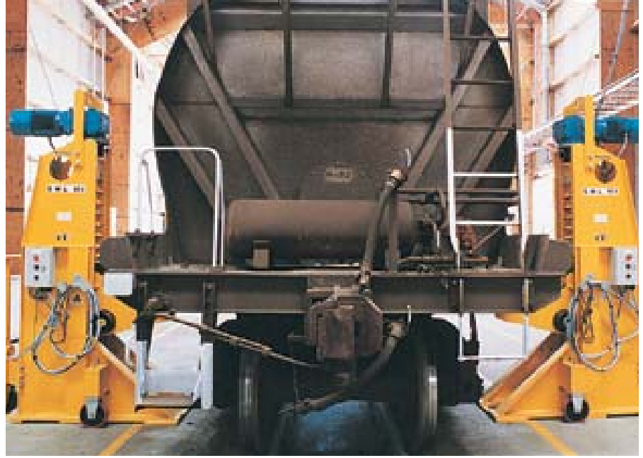
A 40 tonne wagon ready to be lifted at Albany, Western Australia.
