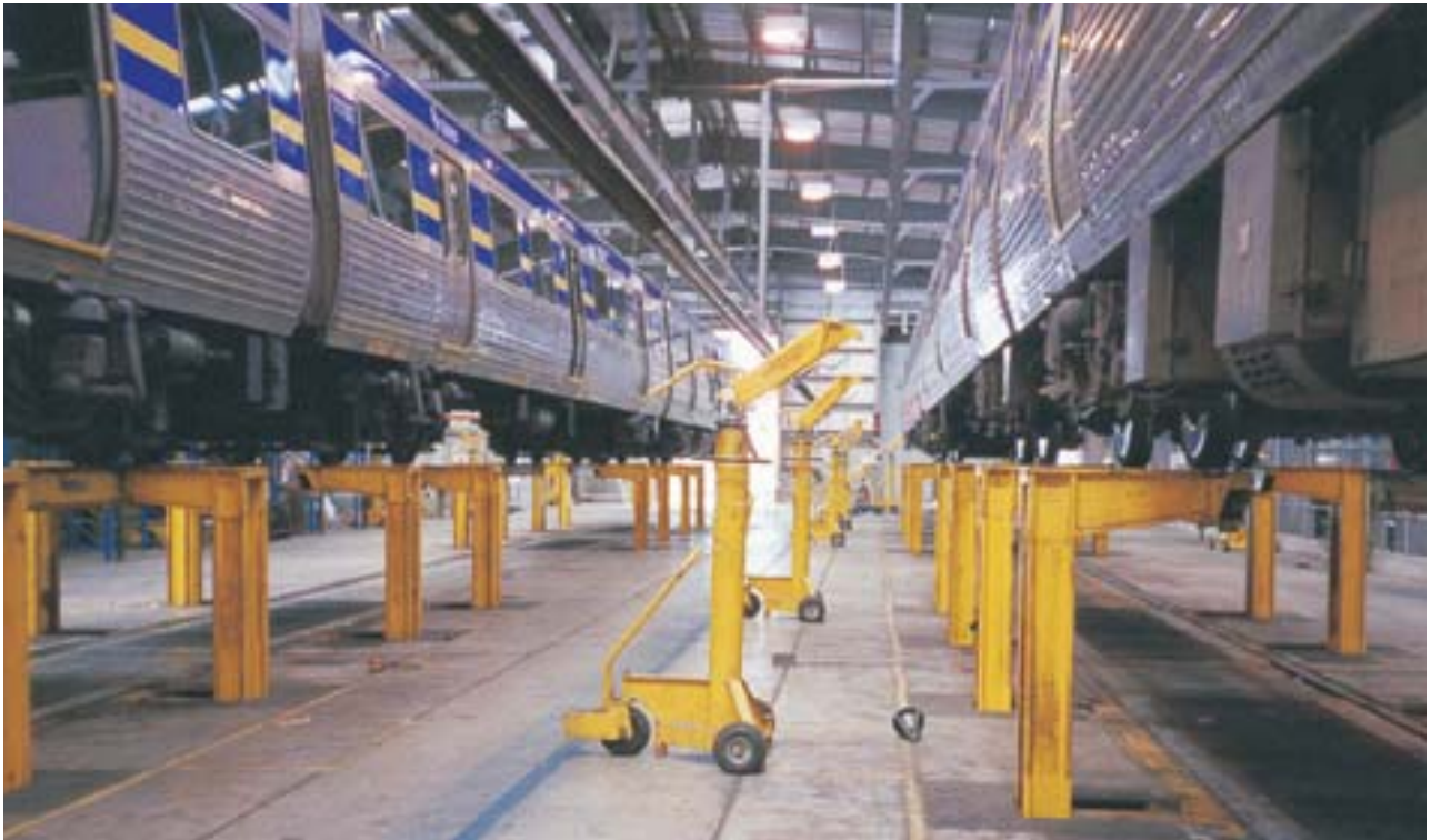
These photos were taken at the Epping service facility in Melbourne, Victoria and show Vector's four car under floor lifting system with special mobile body supports.
